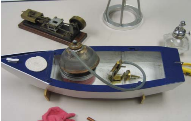
Here are three examples of Gary's handy work: Top Left: Inline 4 cylinder with reversing valve Top Right: Hand (heat) powered Sterling engine Bottom Left: Single acting engine, the "boiler" is a can of sterno and an modified oil can.
